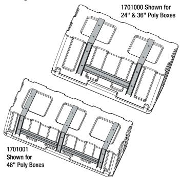
Mounting brackets to be placed on 18" centers for proper installation of the cross brace.
