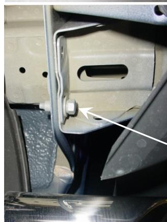
Side view underneath vehicle showing plastic push rivet removed from bumper support bracket. This allows you to pull bumper cover back for better hand and wrench access.
