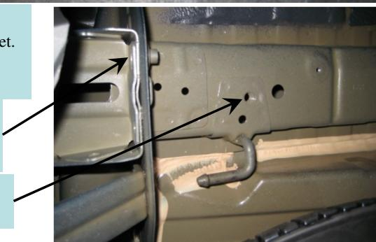
Tighten 8mm-1.25 Gr. 9.8 bolts with torque wrench to 25 Lb.-Ft. (34 N\*M)      Tighten 10mm-1.25 Gr. 8.8 bolts with torque wrench to 42 Lb.-Ft. (57 N\*M)
