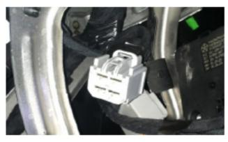
1. Locate and connect the vehicle's 4 pin plug with the matching brake control 4 pin plug. It's found under the dash on the driver's side.
