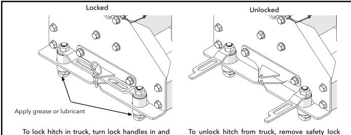
pins and turn lock handles straight out.
