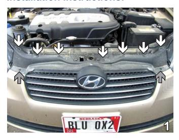
Remove seven Phillips pushpins from the top of radiator cover (see white arrows). Using the 10mm socket, remove two metric bolts (see grey arrows) from radiator cover and lift to remove. Set bolts, pushpins and radiator cover aside to be reinstalled later.
