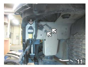
11. On the driver's side, remove the electrical grounds (see white arrows) and move out of the way for baseplate installation. Using the 6mm socket, remove the metric bolt from the air bag sensor (see grey arrow) and move sensor out of way. Set bolt aside to be reinstalled later.
