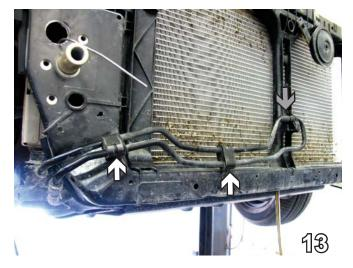
13. Bend coolant line brackets (see white arrows) upward toward radiator to make room for baseplate installation. Using zip ties, secure the bushing of upper section of coolant line (see grey arrow) to cross member of the radiator support bar.
