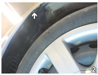
Using the 8mm socket, remove one metric bolt from edge of fascia, just inside wheel well.
