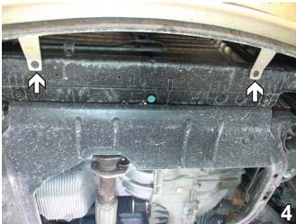
4. Remove two pushpins from the tabs on the bottom center of fascia. Pull upper corners of fascia to the side to release from upper two tabs. Do this to both sides of the vehicle. Pull fascia forward to remove. Set pushpins and fascia aside carefully to be reinstalled later.
