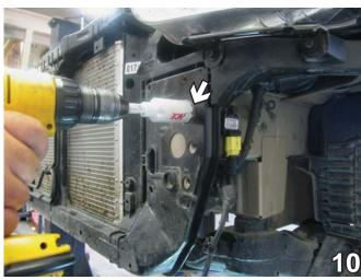
10. Using the 1 1/4" hole saw, drill one hole through the frame end into the frame rail (to insert nut plates later). Note: We recommend spraying the surface with an anti-corrosive paint after drilling. Do this to both sides of the vehicle.
