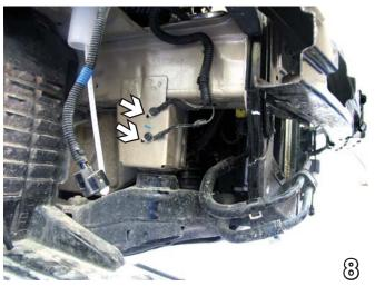
8. On the passenger's side, remove the electrical grounds (see white arrows) and move out of the way for baseplate installation.
