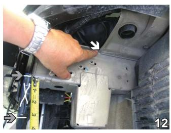
12. Using the reciprocating saw, make a horizontal cut in the radiator support ribbing flush with the bottom of the frame rail. Make another horizontal cut on the radiator support ribbing 3 1/2" down. Using the pliers, flatten the ribbing area between the cuts (see grey arrows). Using the pliers, flatten a 1/2" section of the frame support ribbing where it meets the frame rail (see white arrow). Do this to both sides of the vehicle.
