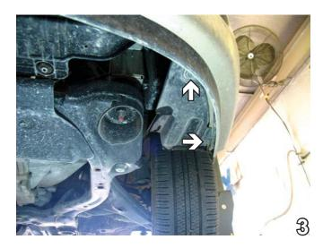
Remove two pushpins from the bottom corner of fascia. Do this to both side of the vehicle. Set pushpins aside to be reinstalled later.
