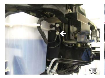
19. On the passenger's side, reinstall washer reservoir using existing bolts. Reconnect electrical grounds to the lower front bolt hole using the #10-16 x 1 self drilling screw (see white arrow).
