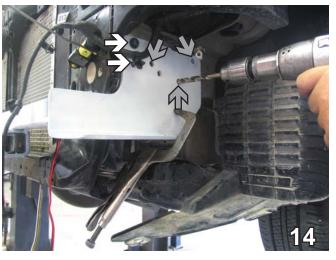
14. On the driver's side, align front two baseplate holes with existing air bag sensor holes (see white arrows). Insert existing bolt from air bag sensor into upper, front hole. Clamp baseplate into place using vise grips. Using baseplate as a template, drill three holes into frame rail with the 13/32" drill bit (see grey arrows). Baseplate painted white for illustration. Actual baseplate will be powder-coat black.
