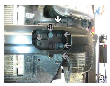
9. Using the 10mm socket, remove one metric bolt from top section of metal bumper bracket (see white arrow). Using the 12mm socket, remove five metric bolts from the metal bumper bracket (see grey arrows). Do this to both sides of the vehicle. Pull metal bumper bracket forward to remove. Set bolts, metal bumper and bracket aside to reinstall later.
