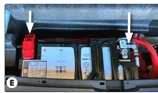
8. Route the T-One® Connector end with **green** wire through the opening and under the metal cargo hook rails. Route along the vehicle's battery and up through the opening under the passenger's cargo rail.
