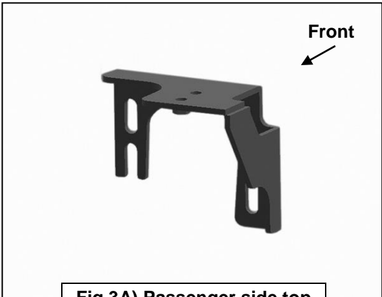
Fig 3A) Passenger side top frame bracket illustrated
