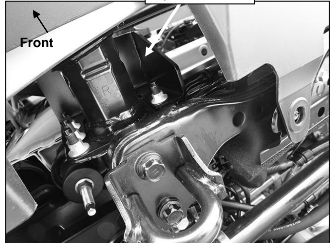
(Fig 4) Reuse factory hex nuts to secure Top Bracket to end of frame. Remove tow hooks
