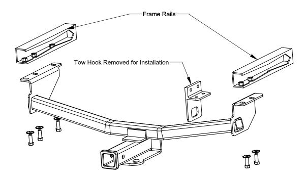
Note: Some models are equipped with appearance panels that cover the frame rails. Prior to installation remove the appearance panels. Return panels and plastic push pin fasteners to the vehicle owner.
